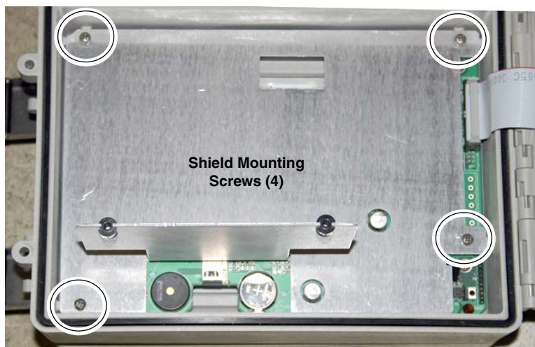
Figure 5-8 Remove non-bubbler shield
