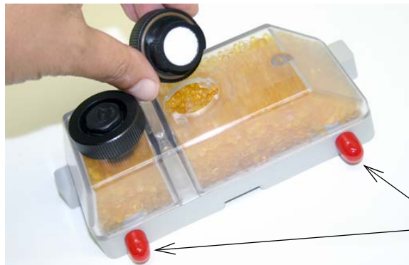
Figure 5-7 Opening the desiccant cartridge chambers
