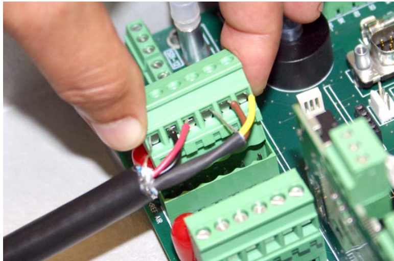
Figure 3-10 Attach wired terminal strip to connector case socket
