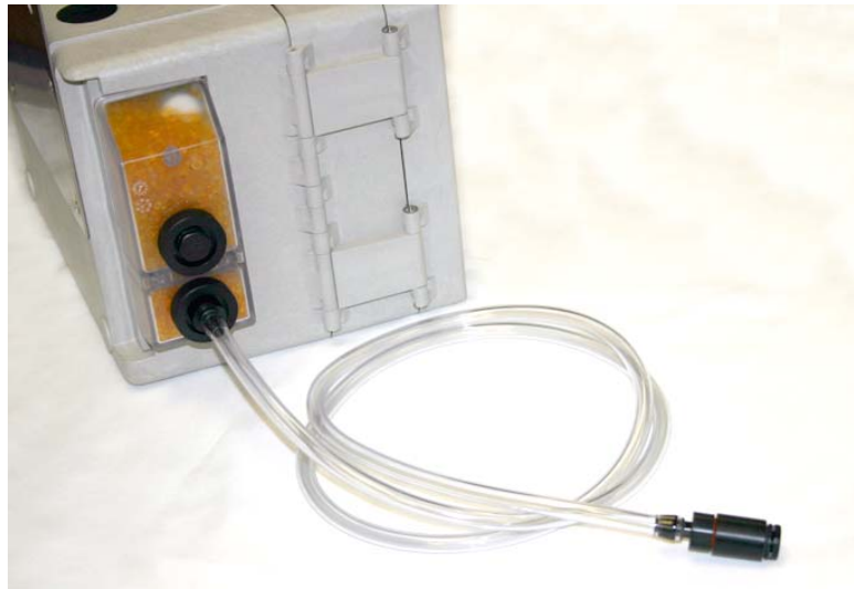
Figure 4-19 Reference port kit: Installed on flow meter
