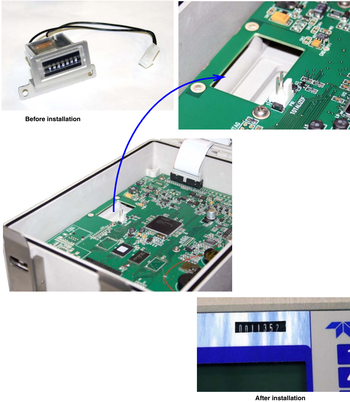
Figure 4-10 Optional non-resettable totalizer installation
