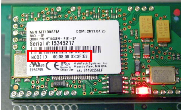
Figure 4-23 Locating the NODE ID (MAC address) on the ethernet modem
