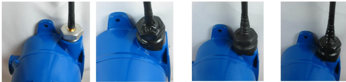
Figure 64 Water-proofing Antenna Connections
