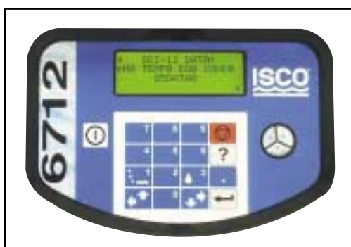
The 6712 Controller is an SDI-12 logger. Manual pump operations are now located on the front panel keys.
