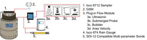
Configuration example: stormwater monitoring using 700 Series flow module
