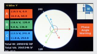
Wiring connections can be checked through the color phasor diagram.
