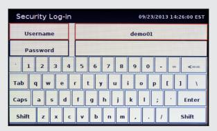
Operating the JEMStar II is simplified with the color display, which provides a user menu for viewing and editing the meter configurations.
