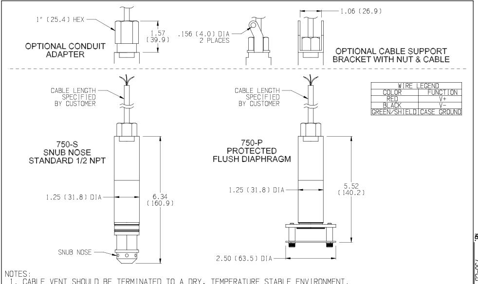
1. CABLE VENT SHOULD BE TERMINATED TO A DRY, TEMPERATURE STABLE ENVIRONMENT. 2. A FUSED OR CURRENT LIMITED DC POWER SOURCE IS RECOMMENDED TO PREVENT DAMAGE DURING FAULT CONDITIONS.
