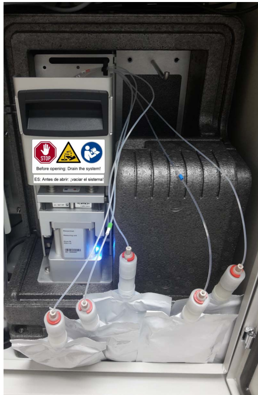
figure 5-7 ChemBags removed to be exchanged
