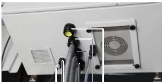
figure 3-24 Connections at the housing bottom (from below) Example: 2 sample channels, 1 drain
