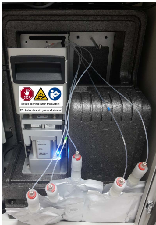
figure 5-19 ChemBags removed from the supporting rod
