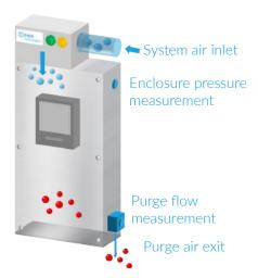
**Purge:** The purge system supplies clean, dry instrument air to the enclosure at a high flow rate for a pre-set time, expelling any potentially flammable atmosphere remaining inside. Enclosure pressure and purge flow are monitored. The enclosure contents are not energised.
