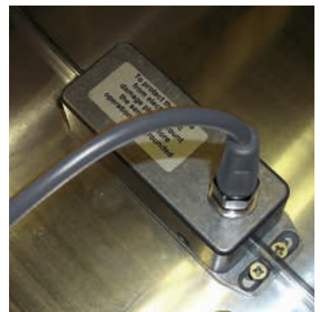
CLAMP-ON SENSOR MOUNTING
