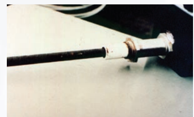
Sensor performance is unaffected by product build-up on sensing rod
