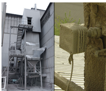
Damp cement mill monitored utilizing a fully insulated sensor
