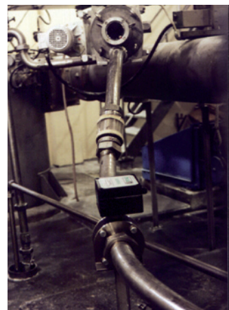
Installation monitoring and reporting the flow rate of powdered materials
