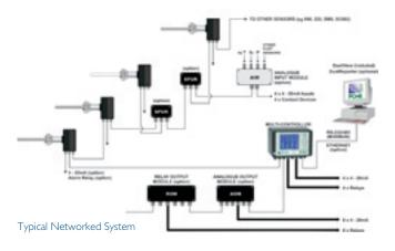
Wood processing facilities normally employ multiple filters often in remote parts of the plant. To monitor these bag houses and cyclones, PCME provide a wide range of Electrodynamic instruments ranging from single channel units to multi-channel systems. These sensors use modbus technology to network to a single control unit. The control unit logs historical data for environmental reporting and process control, displays emission values and allows easy configuration of the system.
