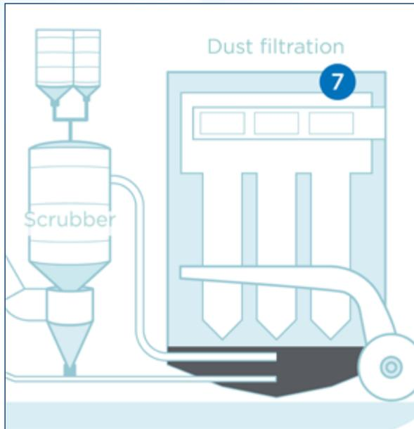
To ensure baghouses are working under optimum performance conditions, the installation of dust monitors to continuously monitor and display particulate emissions provides valuable feedback on filter plant performance.
