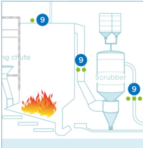
Incineration has a number of outputs such as the ash and the emission to the atmosphere of flue gas. Before the flue gas cleaning system, if installed, the flue gases may contain particulate matter, heavy metals, dioxins, furans, sulfur dioxide, and hydrochloric acid. If plants have inadequate flue gas cleaning, these outputs may add a significant pollution component to stack emissions.
