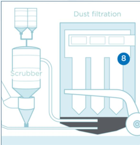
The ability to predict and identify which bag filter row or chamber is likely to fail enables plant operators to achieve maximum service life from filters, reduce maintenance and increase production time while reducing and controlling the potential for large-scale emission events and the associated environmental impact.
