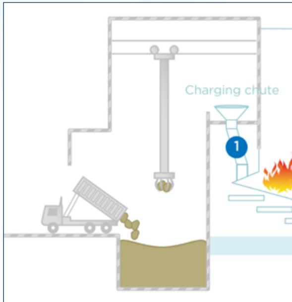
Waste recycling in incineration plants starts with the delivery and incineration of waste. The waste reaches the combustion chamber via a falling chute, which is followed by a hydraulic feed device. To guarantee a constant incineration process, the falling chute has to be filled constantly.
