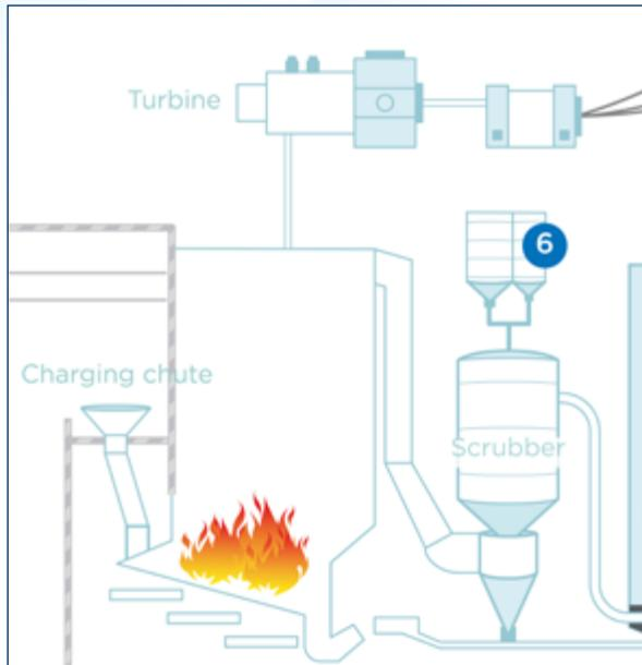
Reagents for the flue gas cleaning such as hydrated lime or activated carbon are stored in silos.
