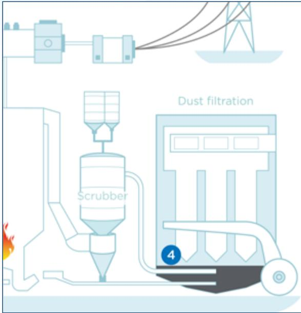
All dust from the filters will fall down into the filter outlets. It is important to avoid a material bridge building up above the rotary valve in the outlet. If such bridging is not recognized the material will build up into the filter and probably plugs it.
