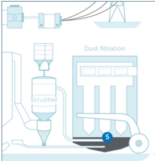
Ash transportation in most cases is done by air slides systems. It is essential to ensure material flow inside the transportation system. Any plugging or interruption in the material flow must be avoided.
