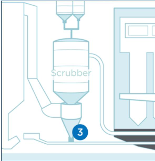
Cyclones are used to separate solids from the gas flow, for example after scrubbers.
