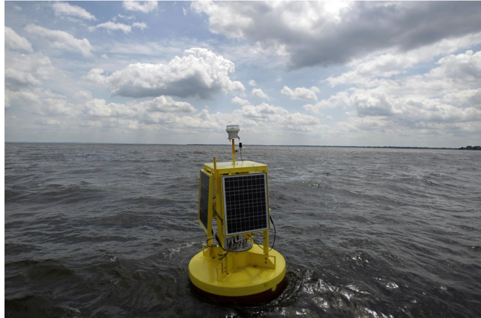
Teledyne Isco 6712 portable sampler attached to a buoy in Lake Winnebago
