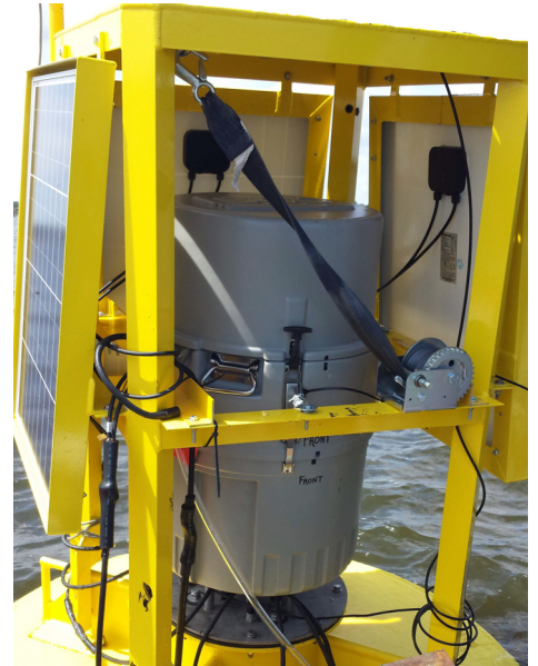
Sampler on buoy with solar panels
