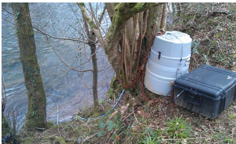
The 3700 Portable Automatic Sampler and the 2150 Area Velocity Flow module deployed together on the River Kensey
