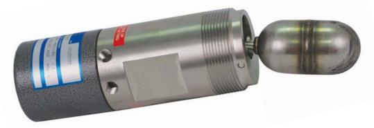
The float moves a magnet into the field of a magnetically actuated pneumatic valve. The pneumatic valve is pilot operated. An amplifying relay provides quick response.
