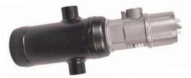
When the liquid rises, the float extension arm moves a magnet which repels an internal magnet de-actuating a microswitch. When the liquid level falls, the float extension arm moves the magnet in the opposite direction, actuating the microswitch.
