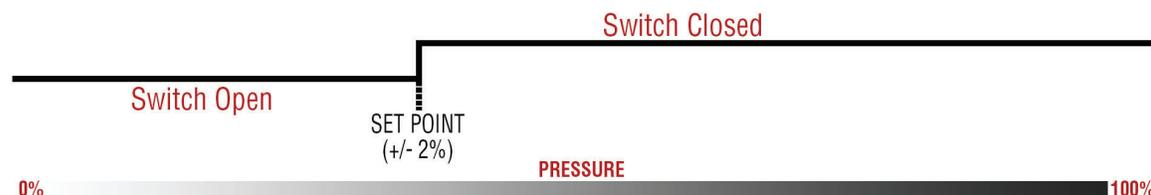
In this configuration, the switch output will be open for pressures less than the selected setpoint. The switch output would then be closed for pressures greater than the setpoint.
