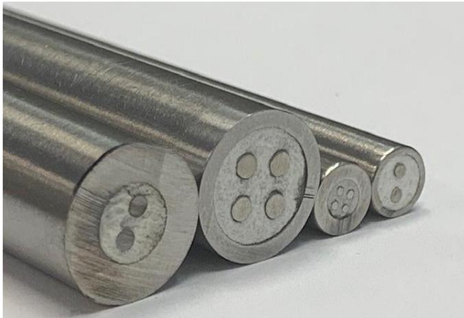
use heavy wall Mineral Insulated cable (MI cable) to limit degradation of the conductors inside and provide better durability. Further robustness is achieved by using thicker elements with larger conductors which have a longer life cycle in extremely harsh environments, though it comes at the cost of reduced flexibility.
