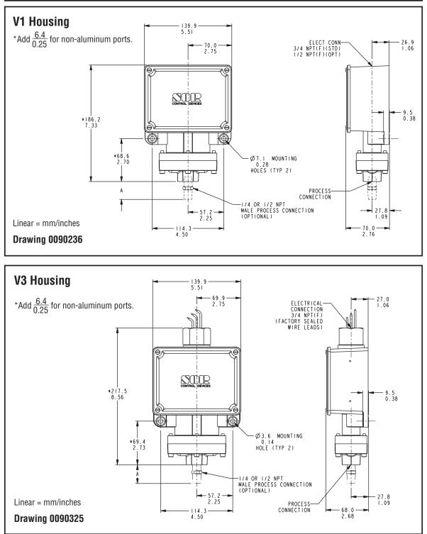
Dimensions are for reference only. Contact the factory for certified drawings for a particular model number.
