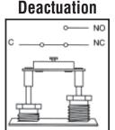
Pressure equal to or less than decreasing set point: Electrical switching element is deactuated.
